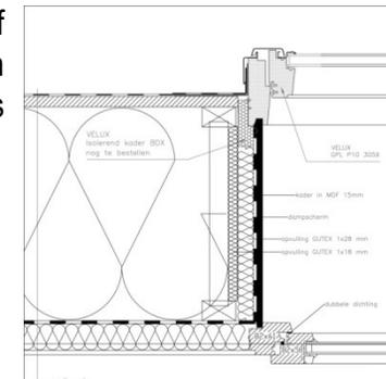
Detail and thermal bridge simulation of the connection between skylight and added inner window.
